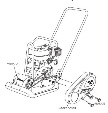
Figure 8. V-Belt Cover Removal
